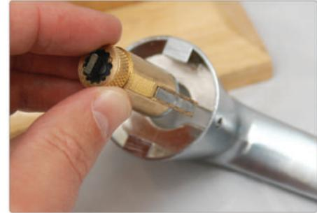
3. Insert the key into the key cylinder from the front of the handle and turn 90° clockwise.
