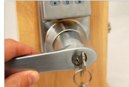
5. Press in both catch pins and snap the rear handle over pins.
