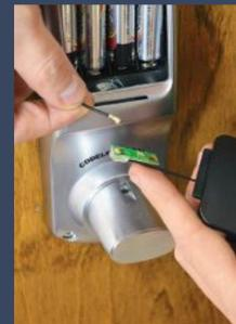
Push the Wifi Connector board into the lock body and fit the battery cover onto the interior lock and secure with screw.
