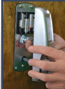
Secure the interior lock body to the door using the 4 socket head screws (2 on top of lock and 2 on bottom).
