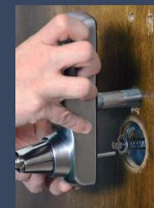
Place the Interior fixing plate over the cable tube and spindle. If cable tube is not used, pass the cables through the opening just below the battery case.
