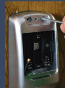
Connect the front lock WiFi cable to the connector board coming off of the battery cover. Once connected, try not to disconnect too frequently as this will loosen the connection.
