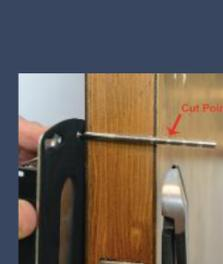
Always cut the bolts at one of the cutting points so as not to damage a thread. Use the cutting edges of pliers to crimp strongly several times around the selected cutting point. If the cut produces a sharp point, please sand the tip of the bolt to smooth it out.
